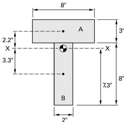
The next task is to transfer the individual moments of inertia about this centroidal axis and add them. To do this, it is helpful to set up a table so all the figures and calculations can be seen easily. This is an especially useful technique when dealing with several individual areas.
